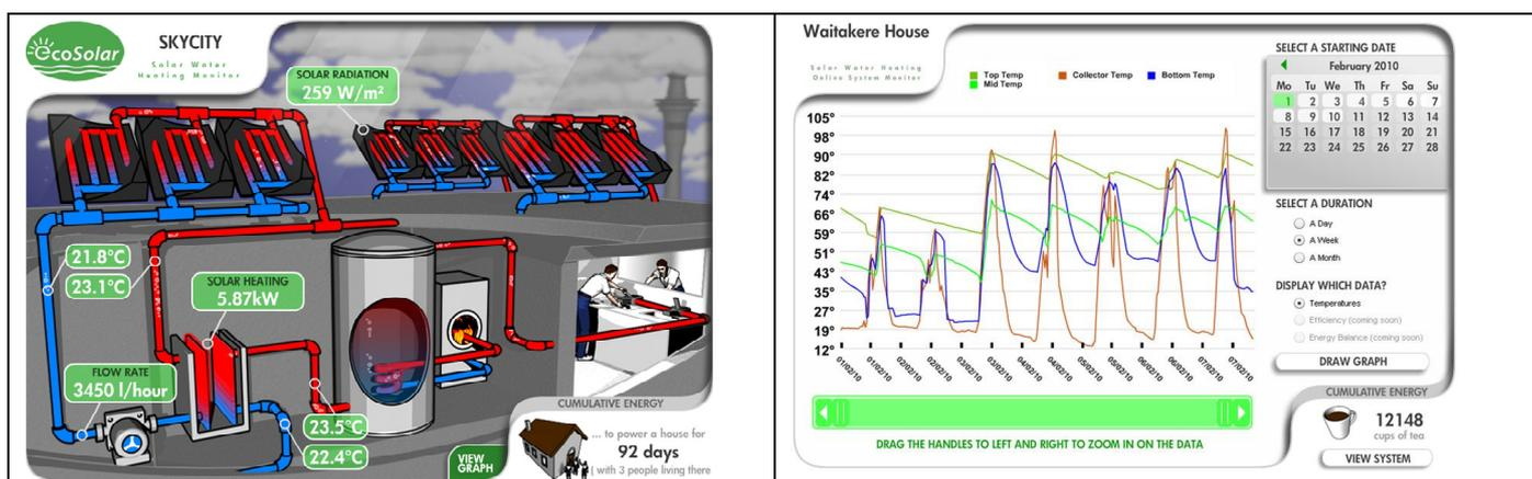
The realtime information displayed depends upon the sensors installed and can be customised to suit each installation, requirements and the expected audience. Solar Monitor is suitable for large, complex, commercial and industrial, as well as domestic scale installations. Realtime information can include;
