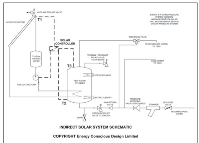
Figure 4: Indirect drainback system utilising a special receiver in the solar circuit. Once the cylinder is up to temperature the pump is turned off and water drains from the collectors.
