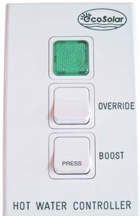
Figure 4 “One Shot” Backup heating controller, allows manual control of the backup heating. The heating is manually turned on and will be automatically turned off, maximising the savings from the solar system.
