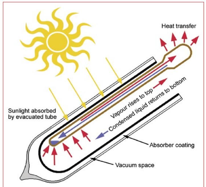
Figure 4: How a heat pipe evacuated tube works
